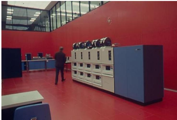
[While we're here, those are a bank of 8 model 2314 disk drives (the 9<sup>th</sup> was a spare) with its Control Unit in blue to the right. Each disk (you can see the canisters that held them resting above the units) held a then massive 25 MB of data. Yes, you read that right. MB, not GB.]
